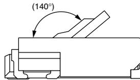
This product has a structure to position an inserted FPC using the FPC tabs. Therefore, insert an FPC at an angle to the board. If the FPC is inserted in the direction parallel to the board, the molded positioning parts block the FPC, leading to incomplete insertion. An FPC inserted at an excessive angle to the board may cause the deformation of metal parts, FPC insertion failures, and FPC circuit breakages.
